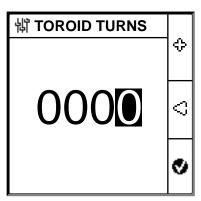
5. Press the button to save the toroid turns. A message **Saved** displays.
